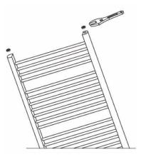
2. Set the position of the wall brackets in relation to the size of your rail approximately 50mm in from each side and mark these positions on the wall in the required location. Use a spirit level to ensure these are horizontally and vertically aligned.
